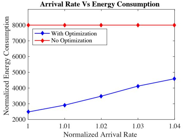
Figure 10: Energy consumption cost with energy optimization and no optimization (Case-4)
