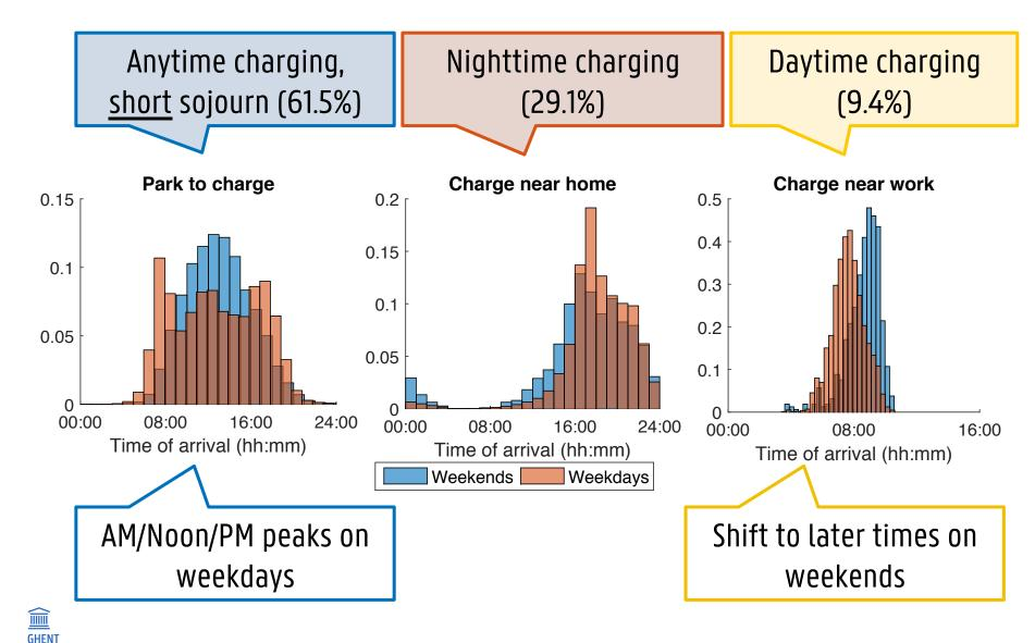
C. Develder, et al., "Quantifying flexibility in EV charging as DR potential: Analysis of two real-world data sets", IEEE SmartGridComm 2016
