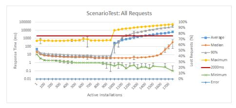
**Fig. 7.** Aggregated results for the test scenario, using JMeter to send data according to the scheme from Figure 6
