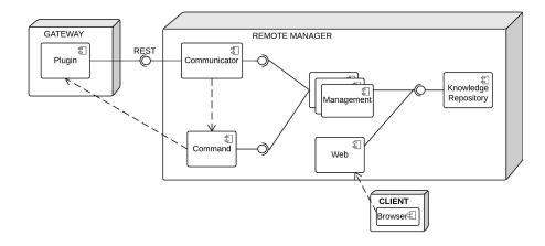
Fig. 4. Architectural Decomposition of the Remote Management System.
