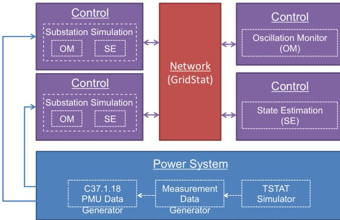
Fig. 8. The GridSim Architecture. The *Power System* component generates PMU measurements that are encapsulated in C37.1.18 data format and forwarded to simulated substations that use real communication middleware (GridStat) to transmit them to OM and SE applications.
