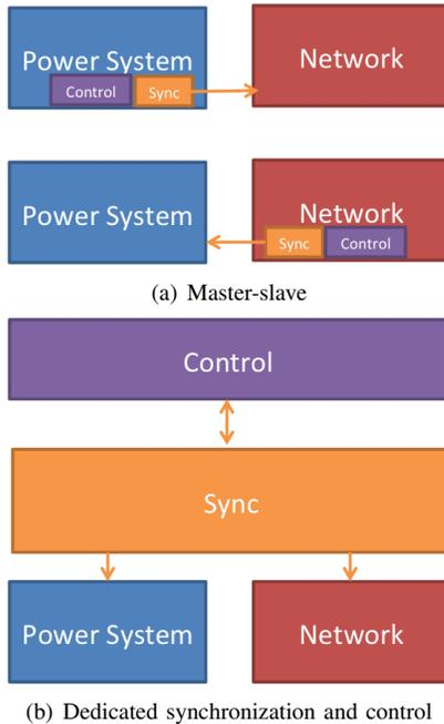
Fig. 16. Two fundamentally different approaches to co-simulation.
