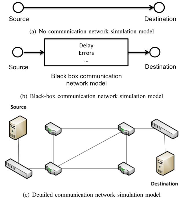
Fig. 15. Level of detail of the communication network simulation model: (a) No communication network simulation model. (b) Black-box: high level abstract simulation model. (c) Detailed communication network simulation model.
