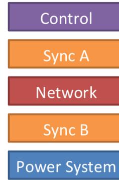
Fig. 17. Layered simulation architecture. *Sync A* is responsible for synchronization between *Control* and *Network* components whereas *Sync B* provides synchronization between the *Power System* and *Network* components. The difference in naming indicates that completely different approaches/technologies may be used.
