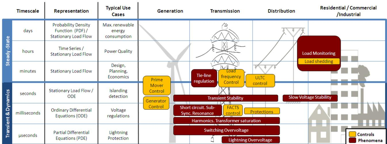
Fig. 4. Time scales of different power phenomena and power control: depending on the time scale, different model representations are adopted. The time scale considered depends on the use case, which typically is related to a particular part of the grid (generation, transmission, distribution, etc.).
