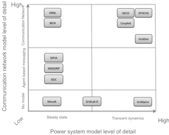
Fig. 14. Classification of smart grid simulators according to supported power grid simulation type and communication network model.
