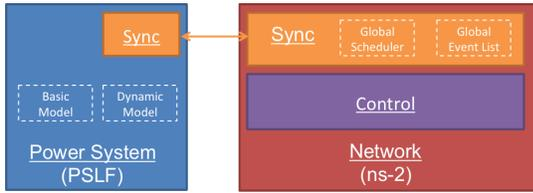
Fig. 6. The GECO Architecture. Power system is simulated by PSLF and state information and control commands are exchanged between PSLF and ns-2 using a bidirectional interface (indicated by *Sync*). Control models (PMU, intelligent agents, etc.) are implemented in ns-2.
