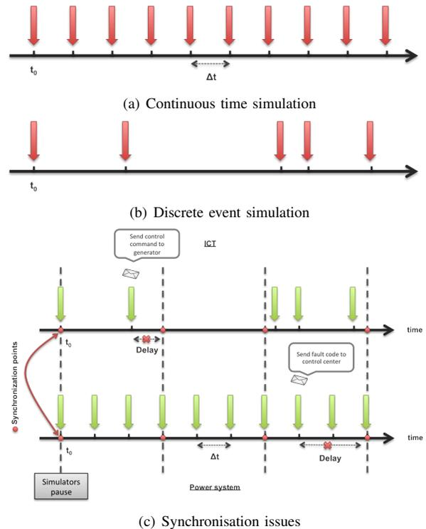
Fig. 2. Continuous time vs discrete event simulation: (a) Time stepped simulation of a continuous time simulation model. (b) Discrete event simulation (DES). (c) Example of simulation errors in an approach based on predefined synchronization points.
