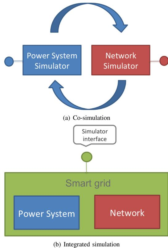
Fig. 1. Conceptual approaches to combining power and communication network simulation: (a) *Co-simulation*: Multiple simulators with specialized tasks, each having their own simulation interface for data input/output, control, etc. The arrows indicate that interaction between the simulators is required. (b) *Integrated or comprehensive simulation*: One combined simulator provides an integrated environment for combined simulation of power system and ICT.
