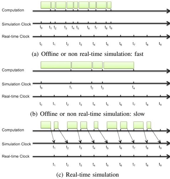
Fig. 3. Non real-time (offline) simulation and real-time simulation: (a) Non real-time simulation in which computation takes less time than the simulated event: simulation clock progresses faster than the real-time clock. (b) Non real-time simulation in which computation takes more time than the simulated event: simulation clock progresses slower than the real-time clock. (c) Real-time simulation: simulation clock and real-time clock are synchronized.
