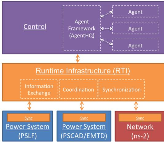
Fig. 7. The EPOCHS Architecture. Intelligent agents implement distributed wide area control and protection schemes. RTI routes all messages between simulation components and manages simulation time.
