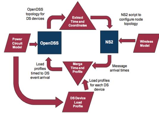
Fig. 5. Example of a co-simulation approach [24].
