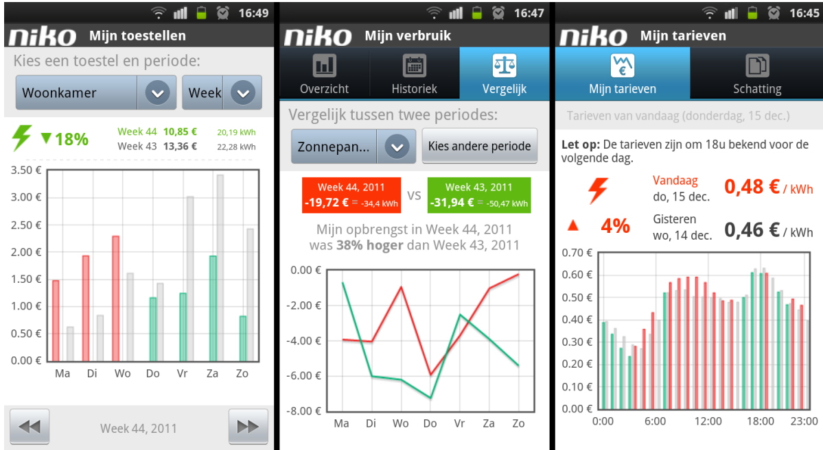
Fig. 6. Some example screenshots of the Android app showing the energy consumption in the living room for this week compared with previous week (left), a comparison of the profit of the solar panels for the last two weeks (middle) and the dynamic tariffs for today and yesterday (right).
