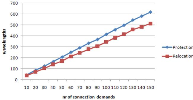
Fig. 6. The comparison in term of the number of wavelengths for protection vs relocation. We see that relocation has an average of about 15% less wavelengths.
