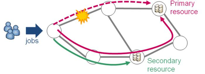
Fig. 1. By relocating to a nearer resource we can create a backup path which a lower number of wavelengths.
