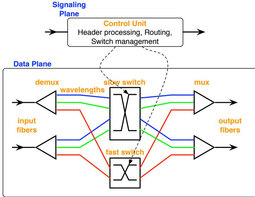
Fig. 2. Multi-granular optical switch supporting wavelength and sub-wavelength switching
