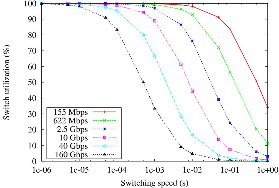
Fig. 1. Upper bound for utilization of an optical switch for different switch speeds and bandwidths (data size is 10 MB)
