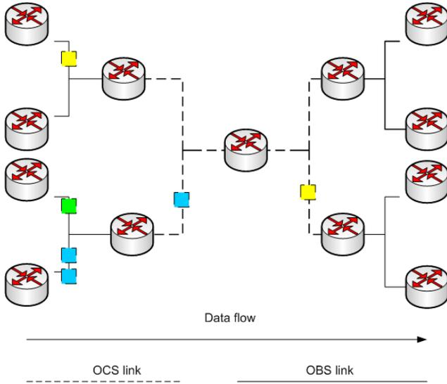
**Figure 2. A  $H_1^4$  topology. Each sub tree has 4 leaf nodes and circuits are put in the core of the network on the first pair of links starting from the core switch.**
