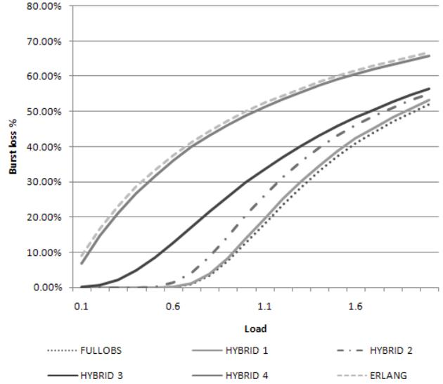
Figure 3. OBS blocking for the different switching techniques
