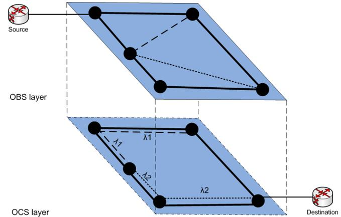
**Figure 1. A client-server hybrid optical switching architecture. The OCS layer presents a virtual topology to the OBS layer where the circuits in the OCS topology are observed as physical links.**
